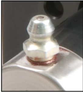
Figure 7.1: A standard grease zerk allows periodic relubrication for Tolomatic IMA Actuators. This can be done without removing the actuator from its installation.
