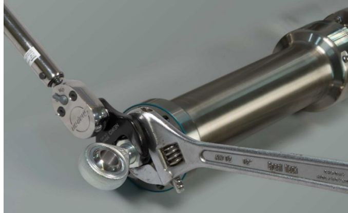
Figure 4.4: For RSH hold the thrust rod stationary using a wrench on the flats at the end of the thrust rod when attaching accessories, linkages or load to the actuator.
