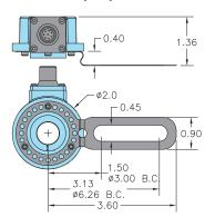
All dimensions are in inches with a tolerance of  $\pm 0.005$ " or  $\pm 0.01$ " unless otherwise specified.
