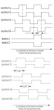
NOTE: ALL DEGREE REFERENCES ARE ELECTRICAL DEGREES WAVEFORM SHOWN WITH OPTIONAL COMPLEMENTARY SIGNALS Ā, Ē, Ž FOR HV AND OD OUTPUTS ONLY.
