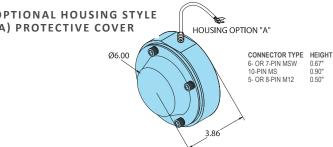
All dimensions are in inches with a tolerance of ±0.005" or ±0.01" unless otherwise specified.
