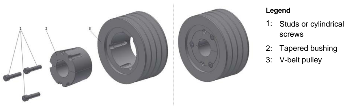
Figure 21: V-belt pulley (disassembled/assembled)
