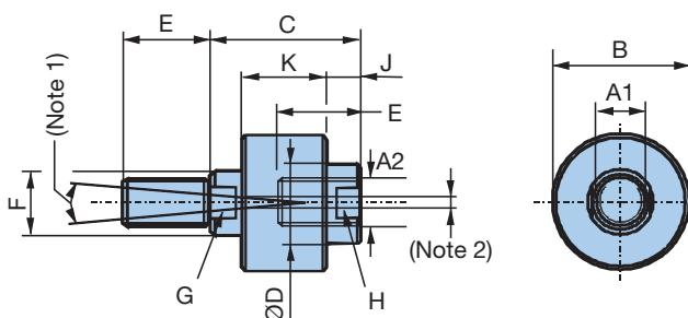
(1) Angle offset  $\pm 5^\circ$  from centerline      (2) Axial offset:  $\pm 1.5$  mm from centerline
