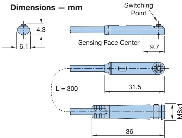
Note: Only PNP logic sensors are compatible with Compax3.
