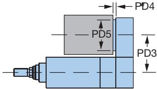
\* PD4 = Flange + Gearhead/overhung load adaptor
