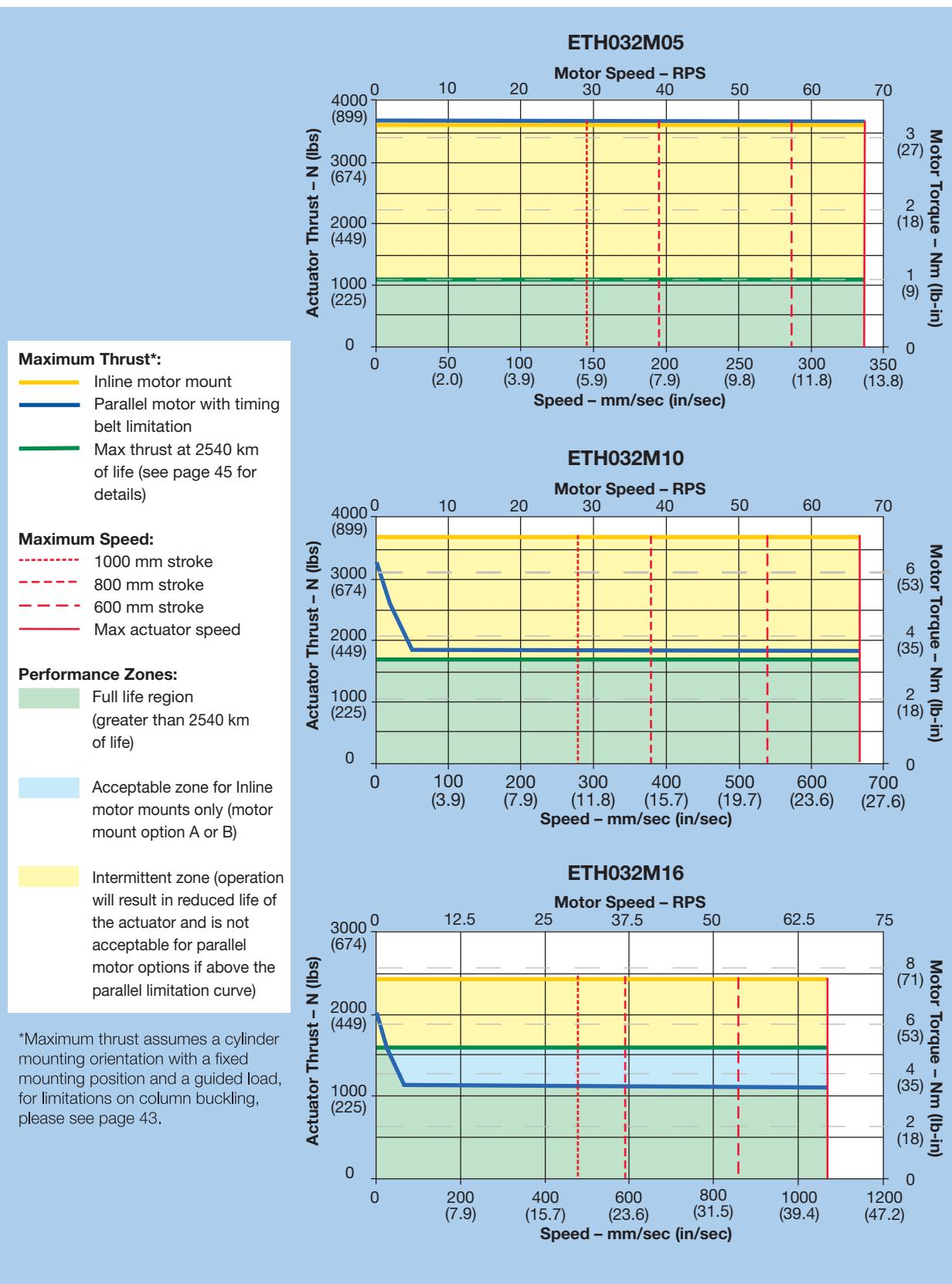
\*Maximum thrust assumes a cylinder mounting orientation with a fixed mounting position and a guided load, for limitations on column buckling, please see page 43.
